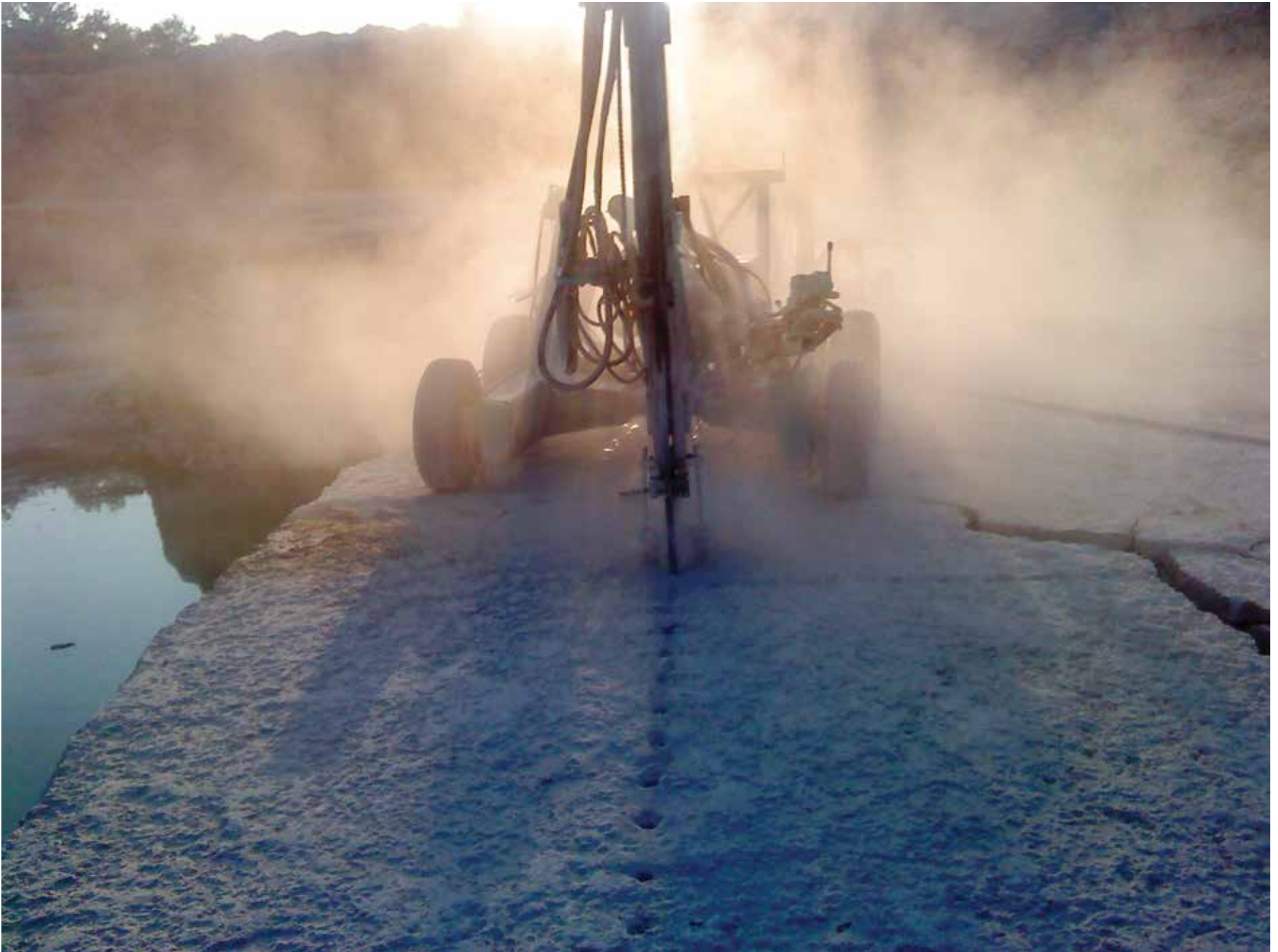
Cutting the stone block
